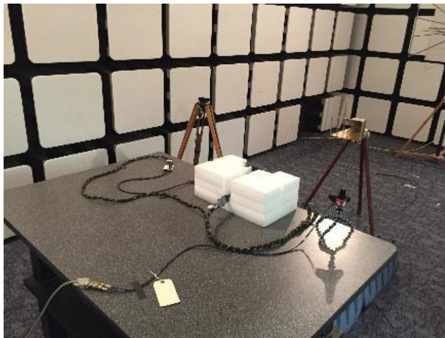
Figure 4 - Radiated Immunity Test Setup -2700 MHz - 6000 MHz Rear
