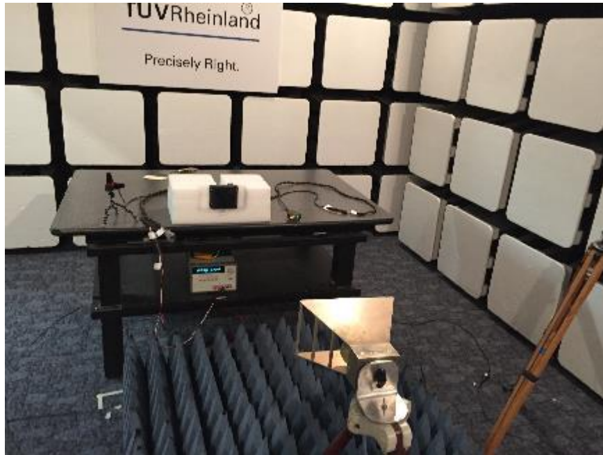
Figure 5 - Radiated Immunity Test Setup Setup - 2700 MHz - 6000 MHz Front
